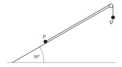
Two particles P and Q are attached to opposite ends of a light inextensible string which passes over a small smooth pulley at the top of a rough plane inclined at 30° to the horizontal. P has mass 0.2 kg and is held at rest on the plane. Q has mass 0.2 kg and hangs freely. The string is taut (see diagram). The coefficient of friction between P and the plane is 0.4. The particle P is released.
