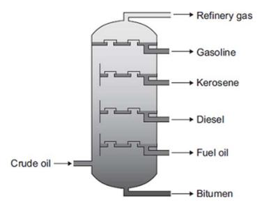
Crude oil is heated until fractions boil off or vaporise. The fractionating tower is hot at the bottom and cool at the top.
